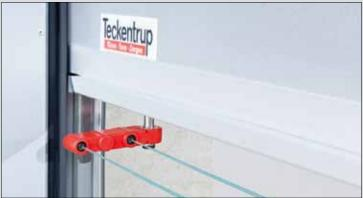
Use of leading light barrier (VL-DUO) for pulse-driven doors. Dual optical sensors ensure that the door reverses if it comes close to an obstacle before actually coming into contact. Being a safety edge mechanism, the VL-DUO satisfies the requirements of safety category E. As such, another light barrier in the passageway is no longer required.
